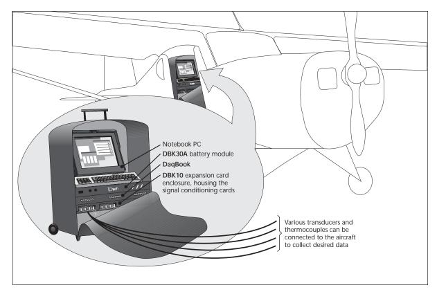
Housed in a soft-sided suitcase, the compact DaqBook data acquisition system is easily wheeled to various test sites and mounted inside aircraft
